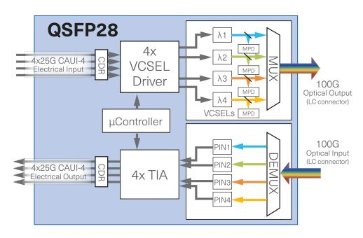
Figure 1: Block Diagram of a 100G SWDM4 QSFP28 Transceiver
